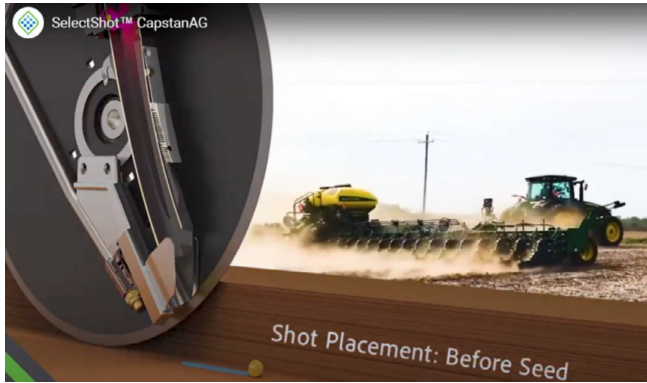
Figure 6. SelectShot (shown above) and 360 Dash technologies pulse liquid products before or on the seed in-furrow. Image credit: CapstanAG.
